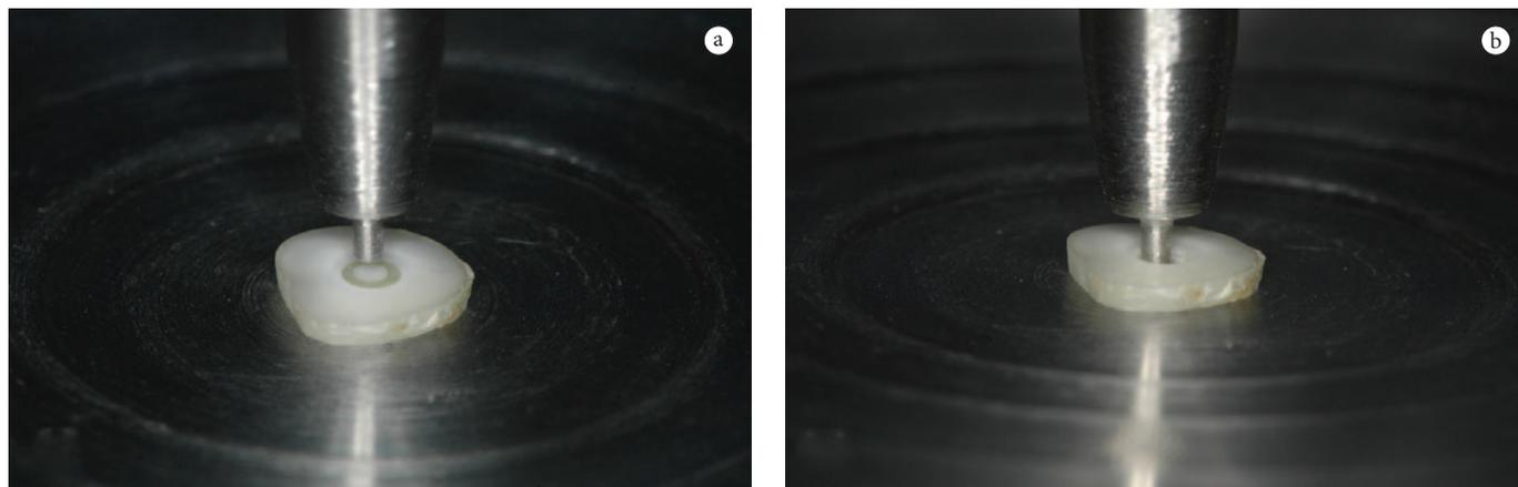
**Figure 1.** a) Slice placed on a holed device to perform the push out tests. See the metal rod device placed on the cemented dowel in the center of the slice; b) Slice after the push out test.
