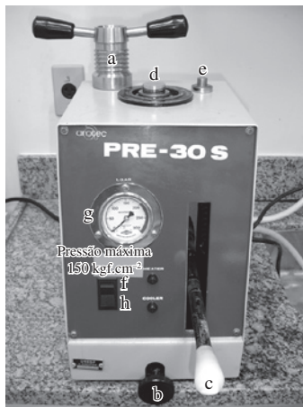
Figure 1. Embedded machine: a) upper cover; b) lock screw; c) handspike; d) metal piston cylinder; e) cylinder cover; f) heating bottom; g) pressure pointer; h) cooling bottom.
