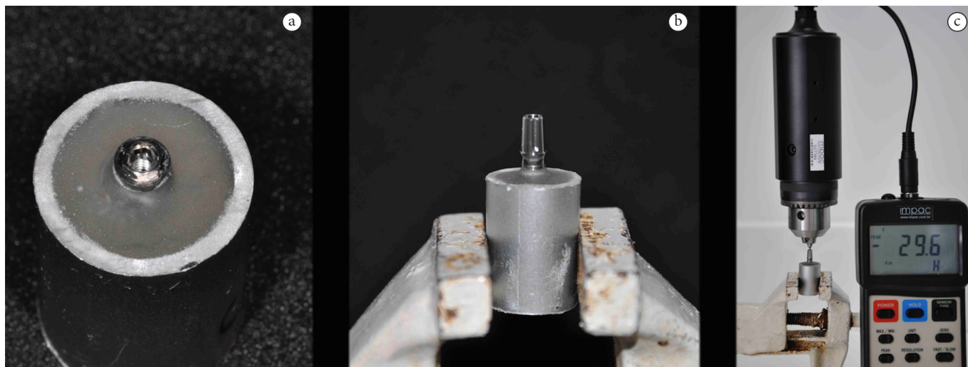
Figure 1. Experimental design: (a) implant submerged in acrylic resin; (b) universal abutments screwed on the implant; and (c) tighten and maintained torque using the digital torque meter.
