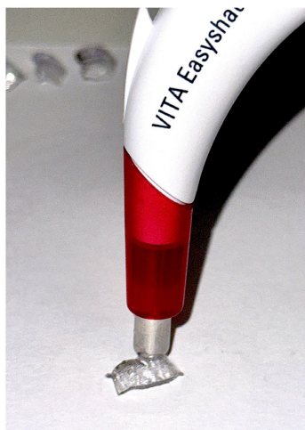
Figure 3. Positioning of the VITA EasyShade Compact spectrophotometer for specimen reading.
