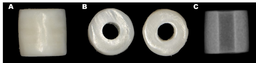
Figure 1. Parameters for fabrication of dentin tubes models. (A) Specimens with a length of 4 mm; (B) Internal diameter of 1.5 mm and wall thickness of approximately 1.0 mm; (C) Digital radiographic images of the dentin tube to confirm the parameters.
