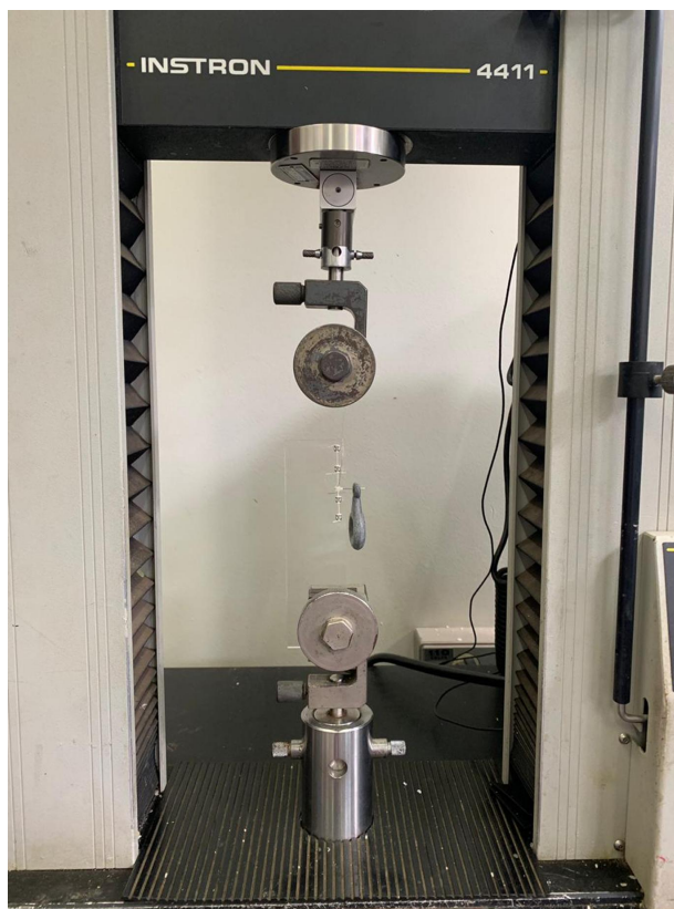
Figure 1. Frictional resistance test on a universal test machine (Instron).
