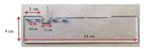
Figure 1. Acrylic plate with brackets positioned for the traction test.
