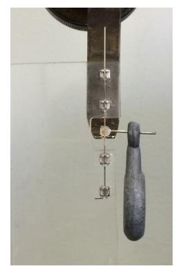
Figure 2. Friction test with conventional metal bracket.
